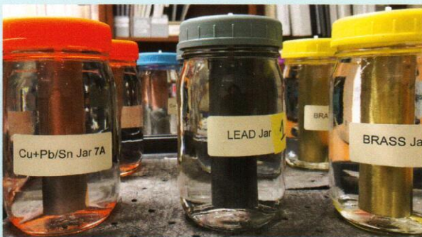
In 2020 and 2021, Water Bureau engineers tested Bull Run water in jars to determine the most effective corrosion treatment to use at the Bull Run Filtration facility
